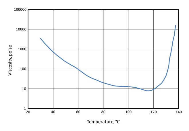
Figure 1 | Viscosity Curve of CYCOM 7668; Viscosity versus Temperature
